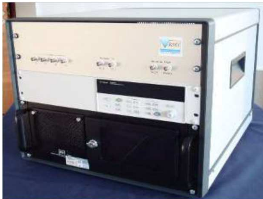
Measurement channel patented for the detection of high energy neutrons
