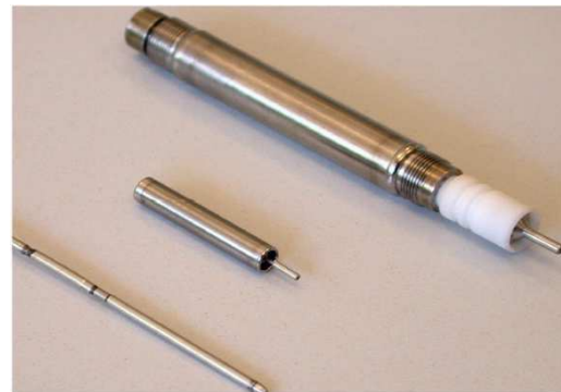
Fission chambers (Diameters: 1.5mm, 4mm, 8mm)
